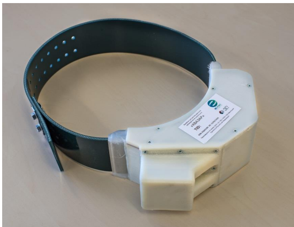
Fig.9. “Quasar” radio collar.
